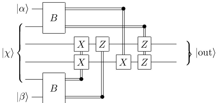
FIGURE 1. Teleporting a CNOT ( $|\text{out}\rangle = \text{CNOT}|\beta\rangle|\alpha\rangle$ ).
